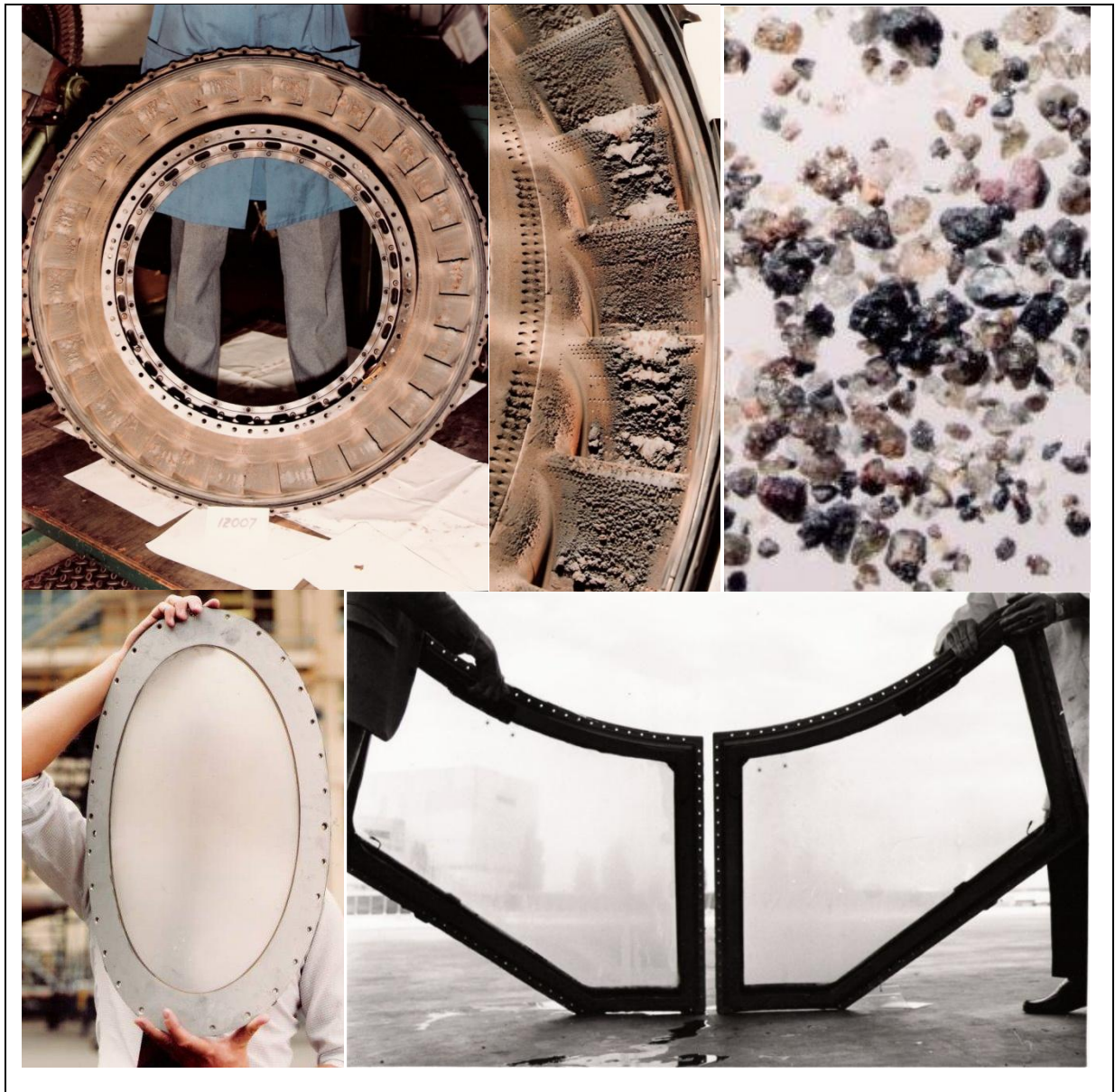
Figure 1 Photographs of damage caused to the British Airways Boeing 747 that encountered ash from the Mt. Galunggung eruption [courtesy Capt. Eric Moody] Top row, from left - Stator blades from turbine; Close up of melted ash on stator blades; Magnified image of ash from pitot system. Bottom row, from left - Lens from landing light windscreen; Windows after washing clean.
